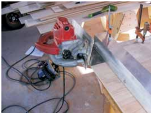
Left—WEST SYSTEM 875 Scarffer™ being used to machine scarf bevel and step.
